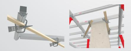
TITAN's patent pending asymmetrical design can also be used with TITAN's Universal Wedge Clamps and 2x4s located on all TITAN jobs. One Wedge Clamp Column Brace pair replaces up to **five 3-post x-braces**. When installed, it has a lateral capacity of 1,780 lbs (2.5:1 FS).
