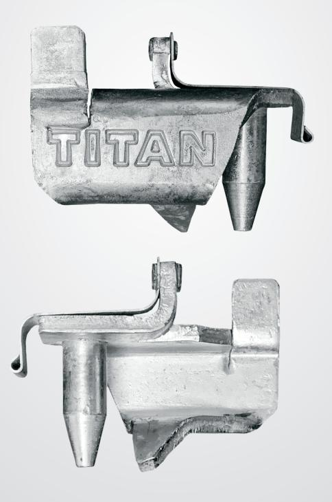
The **XL Clip**, a new creation inspired by the needs of our clients, streamlines the process of extending shores. The standard four-bolt configuration typically used to attach the one meter extension to XL shores can be replaced with only two XL Clips. Load capacity is maintained while the clips are in use and the spring clip feature ensures the device will stay in place when attached. The clip's simple installation and removal requires only a hammer; no wrench or other tools necessary.
