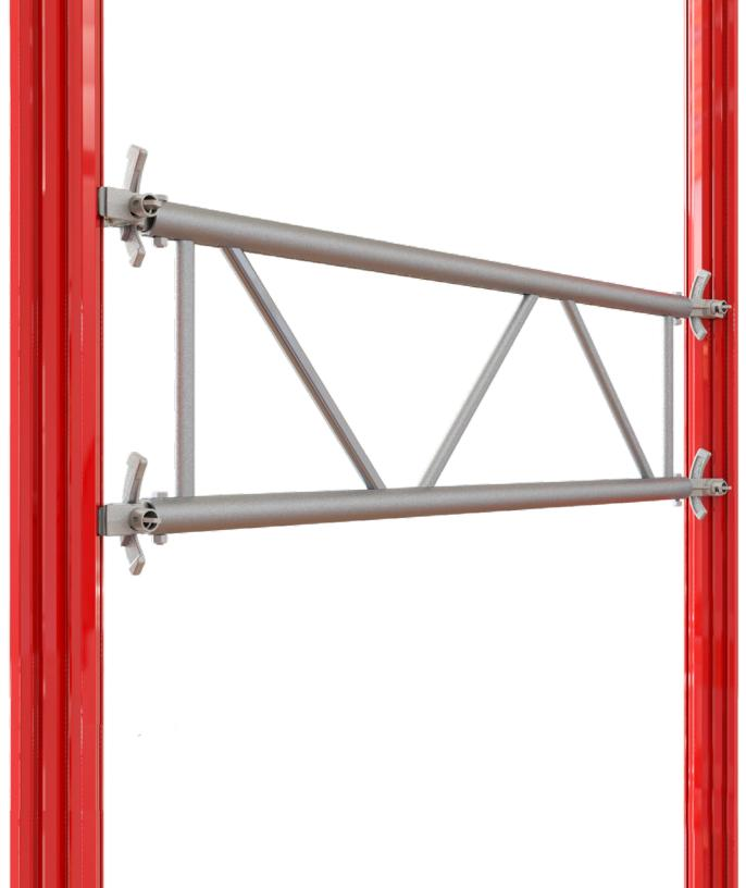
Patented XL Ledger Clamp Our unique XL ledger clamp system uses a 2-staged curved bolt-action style wedge that automatically draws into position and provides improved hammer striking clearance.
